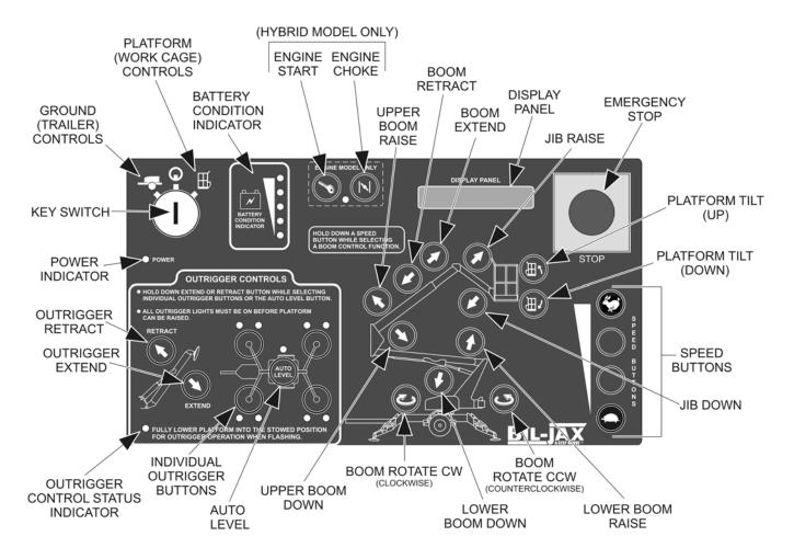
Figure 3-1. Ground Control Station.
